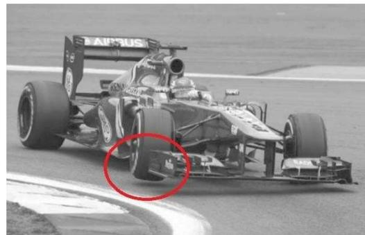
**Figura 7** – Falta de *grip* no pneu dianteiro. Adaptado de *Charles Pic lifting an inner wheel at the 2013 German Grand Prix*. (Seward, 2014).
